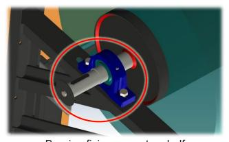
Bearing fixing on motor shelf
